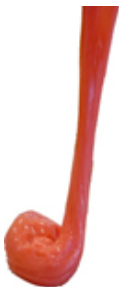
Figure 3: PVA glue, otherwise known as poly(vinyl alcohol), with borax added to form cross-links. Here, the polymer has been allowed to stretch slowly under its own weight.
