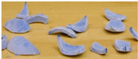
Figure 4: A shattered polymer squash ball – cooling to -196^{\circ}\text{C} resulted in the rubber ball becoming brittle
