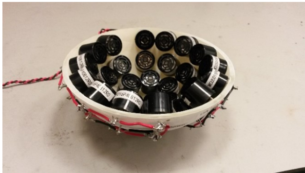
Figure 3: Our sonic tractor beam. Each black transducer is a source of sound waves.
