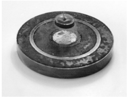
Figure 2: A YBa 2 Cu 3 O 7 superconducting disc being “levitated” by a permanent magnet.
